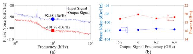
**Fig. 5** (a) Phase noise spectrum of the input 18 GHz microwave signal (blue dashed line) and the frequency divided 6 GHz signal (red solid line). (b) Phase noise at a 10 kHz frequency offset and frequency divided signal power for different input microwave signal frequencies
