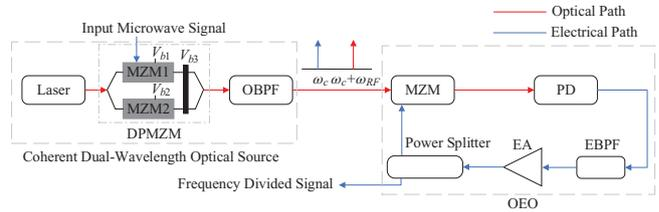
**Fig. 1** Schematic diagram of the proposed one-third frequency divider. DP-MZM: dual-parallel Mach-Zehnder modulator; OBPF: optical bandpass filter; MZM: Mach-Zehnder modulator; PD: photodetector; EA: electronic amplifier; EBPF: electrical bandpass filter
