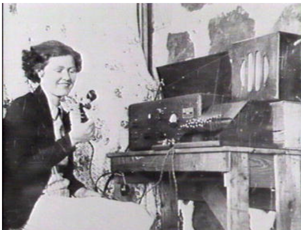
Miss Jessie Chalmers, (later Mrs. Geoff Holt of Delmore Down) daughter of Charles and Cora Chalmers, seated at a pedal wireless set installed at MacDonald Downs by Skipper Partridge and John Flynn. John Flynn made the table out of the case in which Alfred Traeger forwarded the set from Adelaide. Note the stone walls and lime cement. DATE 1936. Source: Picture NT. Photo number: PH0057/0089
