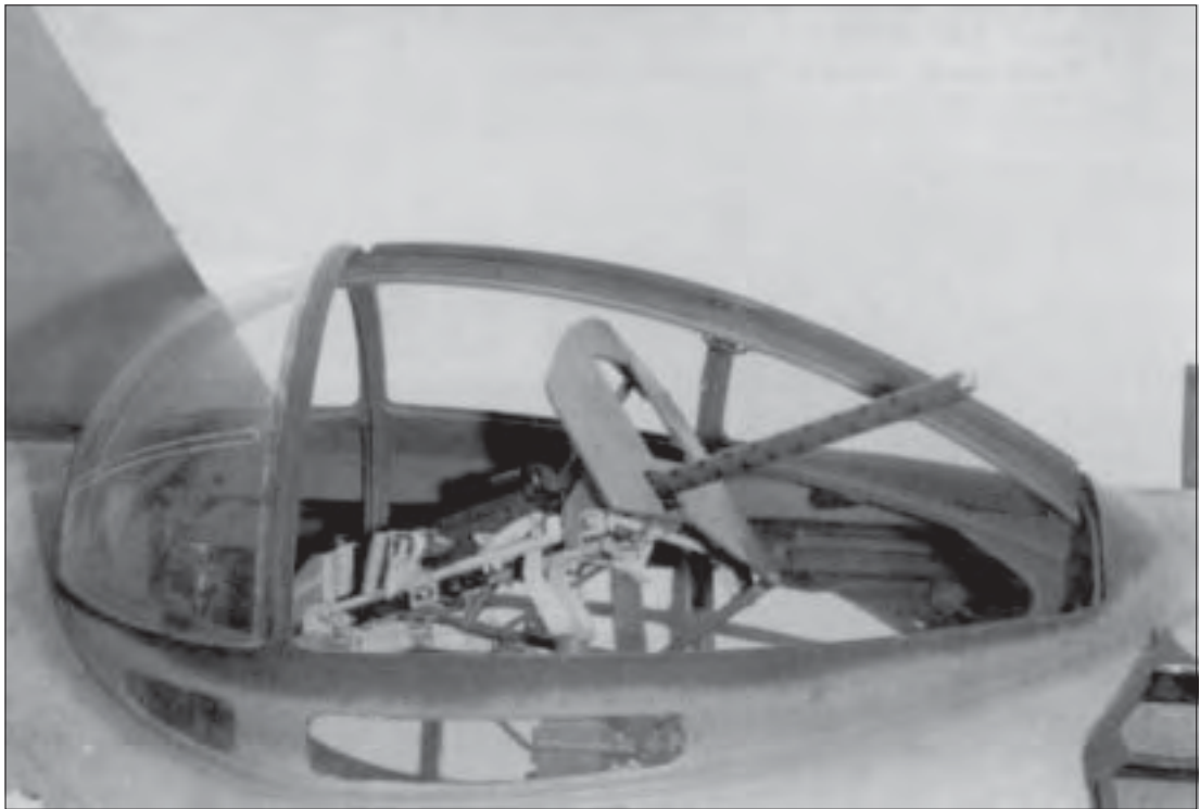
Photo 10. Port waist blister of a PBY-5A with the gun in firing position (Scarborough 1995:23).
