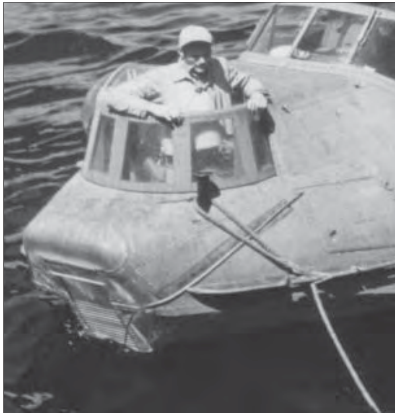
Photo 74. A crew man stands in the forward gun turret awaiting the captain's orders to let go the mooring line on the snubbing post. Note that the gun turret is turned to starboard, to facilitate accesses to the mooring rope (Scarborough 1995:43).
