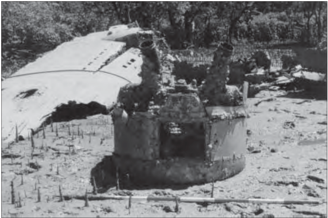
Photo 52. The starboard engine, lying face down at the A24-1 wreck site. Note the exhaust collector ring on the back of the engine. Scale in 20cms (Photo: Jung 1998).
