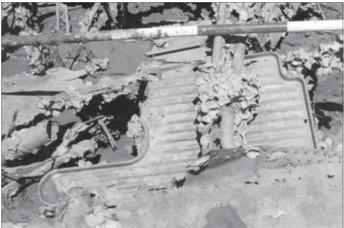
Photo 49. Captain's rudder control pedal inside the A24-1 wreck site cockpit. Scale in 20 cms (Photo: Jung 1998).
