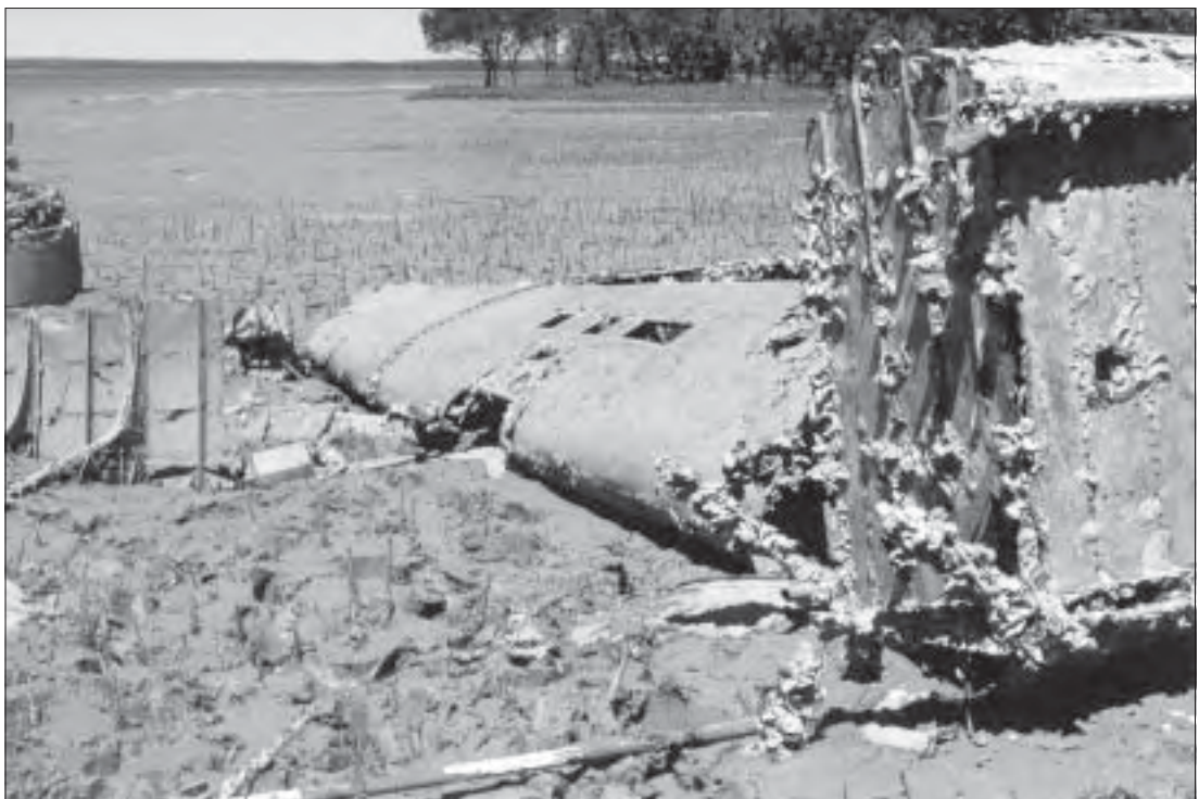
Photo 57. The leading edge of the starboard wing of A24-1. The starboard engine fire wall is visible in foreground (Photo: Jung 1998).
