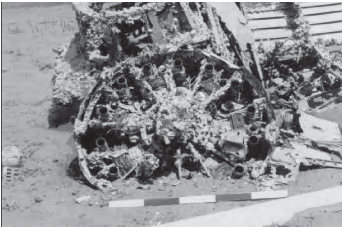
Photo 51. Port engine resting against the bow turret of A24-1. Compared with Photo 48, the exhaust collector ring was removed recently for a museum display. Scale in 20cms (Photo: Jung 2000).
