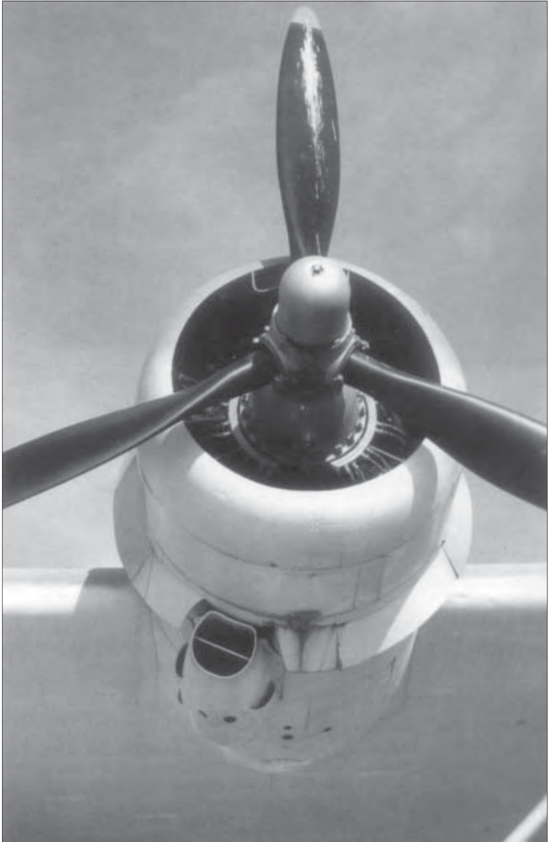
Photo 18. The Pratt & Whitney R-1830-92 engine. Note the oil cooler below the engine to left on the nacelle and the air intake inside the cowling (Kinzey2000:48).
