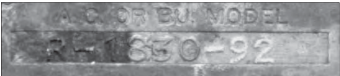
Photo 6. Inset 1 from Figure 5, showing engine type number.
