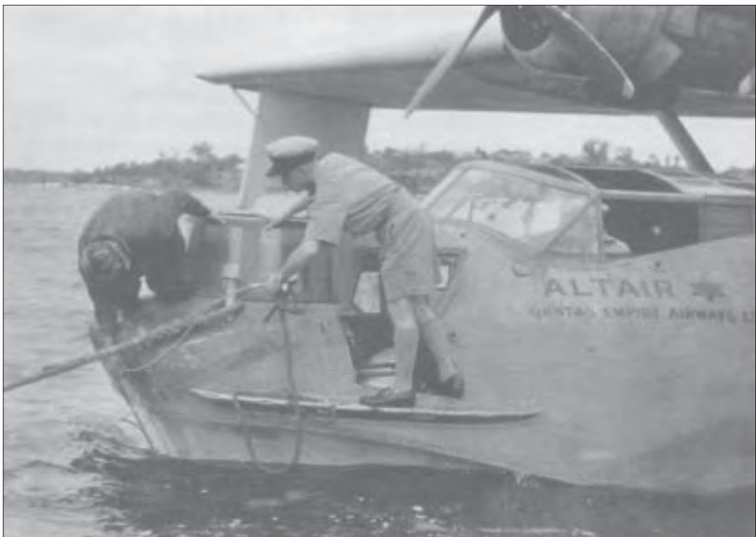
Photo 75. Qantas Catalina 'Altair Star' about to cast off. Note the lizard line attached to the mooring or snubbing post. The crew man to the right is holding the pendant line. The folding anchor is stowed in the anchor locker, at the man's feet (Leebold 1995:41).
