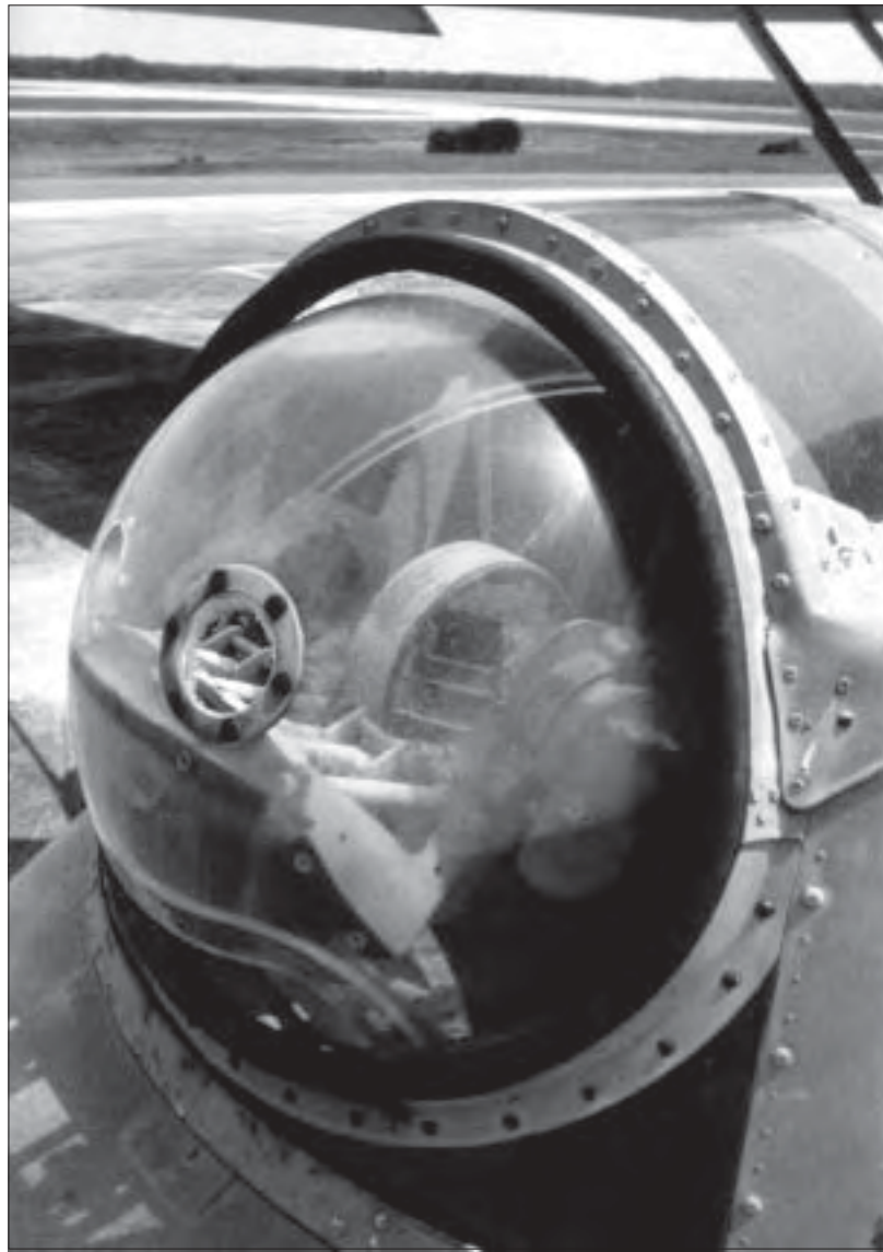
Photo 14. Bug eye turret on the PBY-5A and later Catalina types with twin .30 in. calibre machine guns (Scarborough 1995:16).
