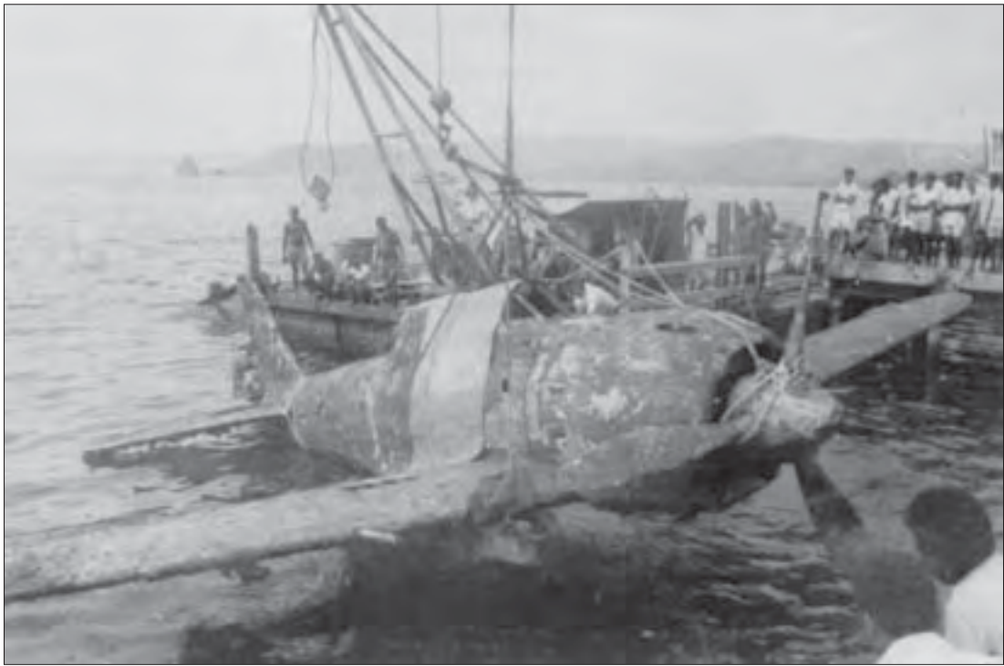
Photo 75. 'An A6M5 Zeke recovered from Simpson Harbor, Rabaul, in 1971...The Zeke was shipped to the USA but neglect of anti-corrosion precautions have since taken their toll to the point where disintegration is now well advanced and the aircraft today is little more than a rather expensive curiosity' (Darby 1979:23).
