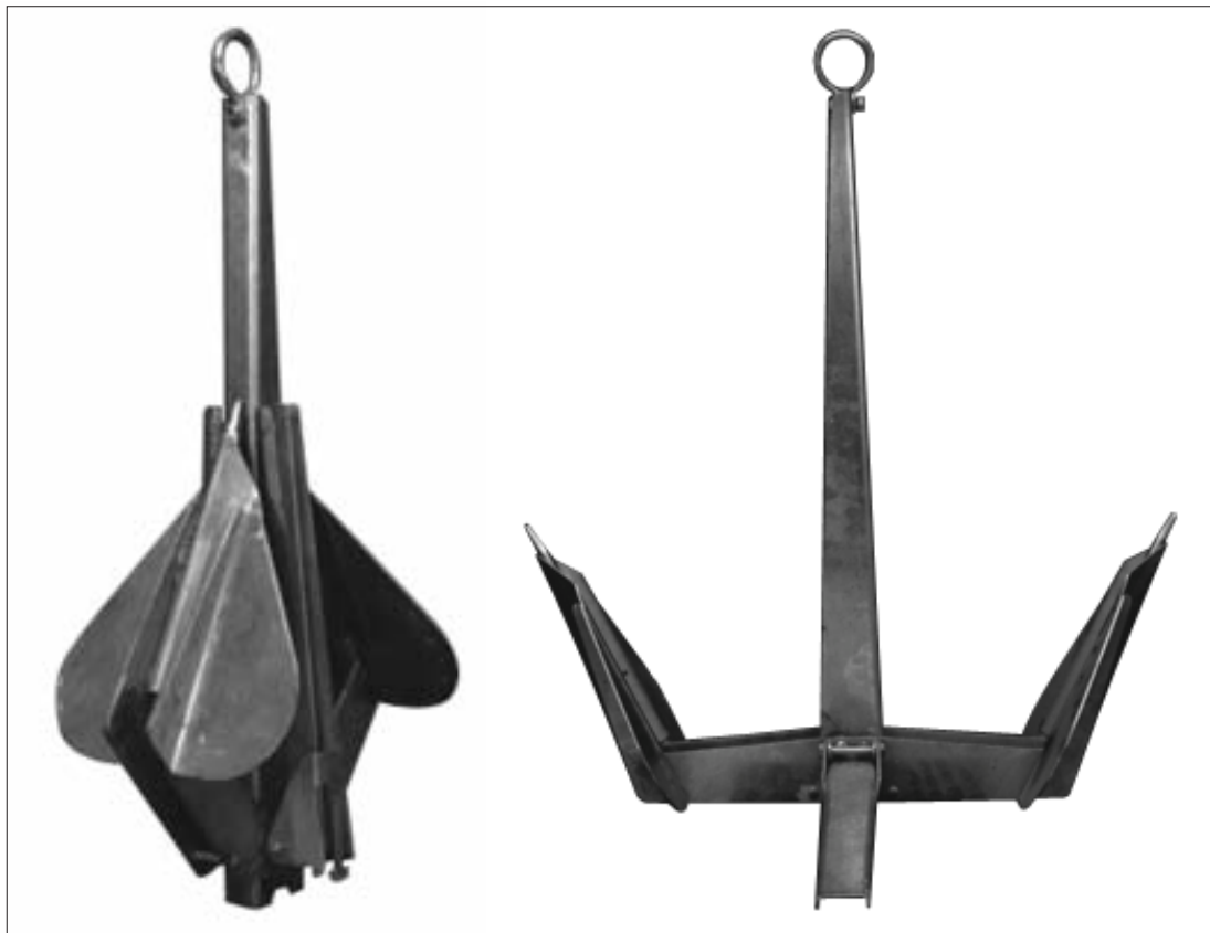
Photo 9. Standard size folding anchor from Catalina 4, folded (left) and extended (right) (Photo: Jung 1995).
