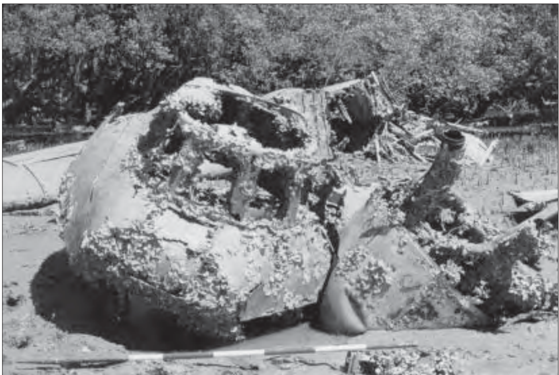
Photo 45. Bow of A24-1 with gun turret. The port engine leans, face down against the fuselage. Note the exhaust collector ring on the engine. Scale in 20cms (Photo: Jung 1998).
