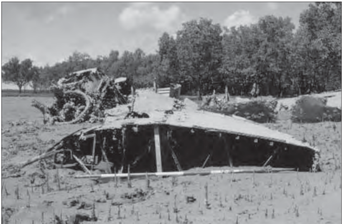
Photo 59. Port wing tip, showing break point of the central wing section from the outer wing section. Scale in 20 cms (Photo: Jung 1998).
