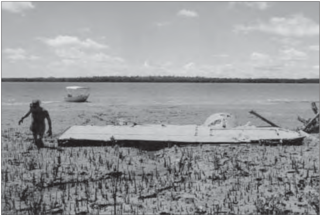
Photo 60. Rear of the port wing of A24-1. The engine cowling rises along the leading edge (Photo: Jung 1998).
