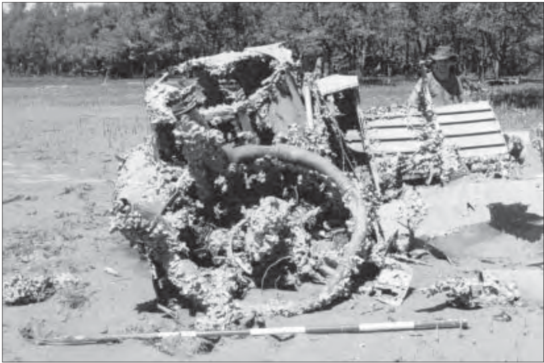
Photo 50. Port bow view of A24-1 with port engine resting against the bow gun turret. Note exhaust collector ring attached to engine. Scale in 20cms (Photo: Jung 1998).
