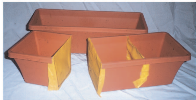
Figure 2. A disassembled microcosm. The three-compartmented planter box is divided by double layers of nylon silk-screen cloth mesh root barriers (45 \mu m pore size). A double layer was cemented into a slot on the right side, and single layers were cemented across each cut end of the completely separated left side. When assembled, the compartmented box nested tightly within the fully-intact outer box, but the separated end periodically could be lifted vertically, sliding the layers of cloth mesh against one another and severing hyphae that crossed them.
